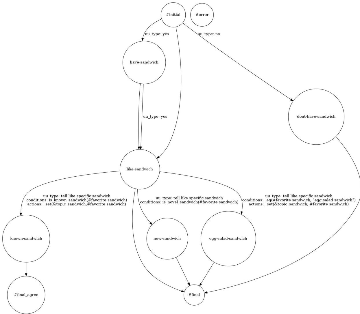
Among the functions used in the conditions of transitions and actions that are executed after transitions, those that are not built-in are defined in `scenario_functions.py`.
