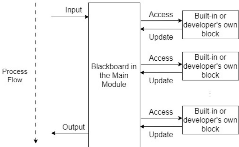
The main module creates and returns a system utterance by making modules called blocks sequentially process the data (including user utterances) inputted at each turn of the dialog. The inputted is data copied to data called blackboard<sup>1</sup> in the main block. Each block takes some of the elements of the blackboard and returns data in dictionary format. The returned data is added to the blackboard. If an element with the same key already exists in the blackboard, it is overwritten.
